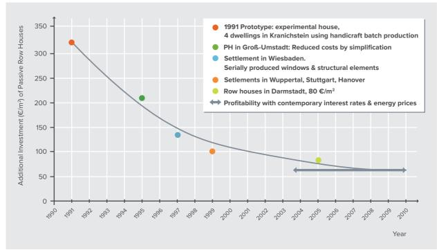
Figure 4: Learning curve showing the progressive decrease in the incremental cost of meeting the passive house standard for the central unit of row houses in Germany. These compare to costs for conventional buildings of ca. €1250 to 1750 per m2.
