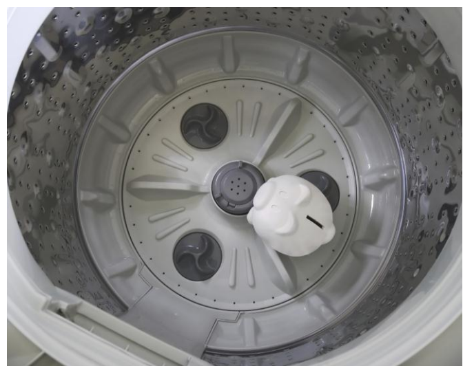
Figure 6: Vertical axis ‘high-efficiency’ washing machine, Impeller, Source: iStockphoto (2013)
