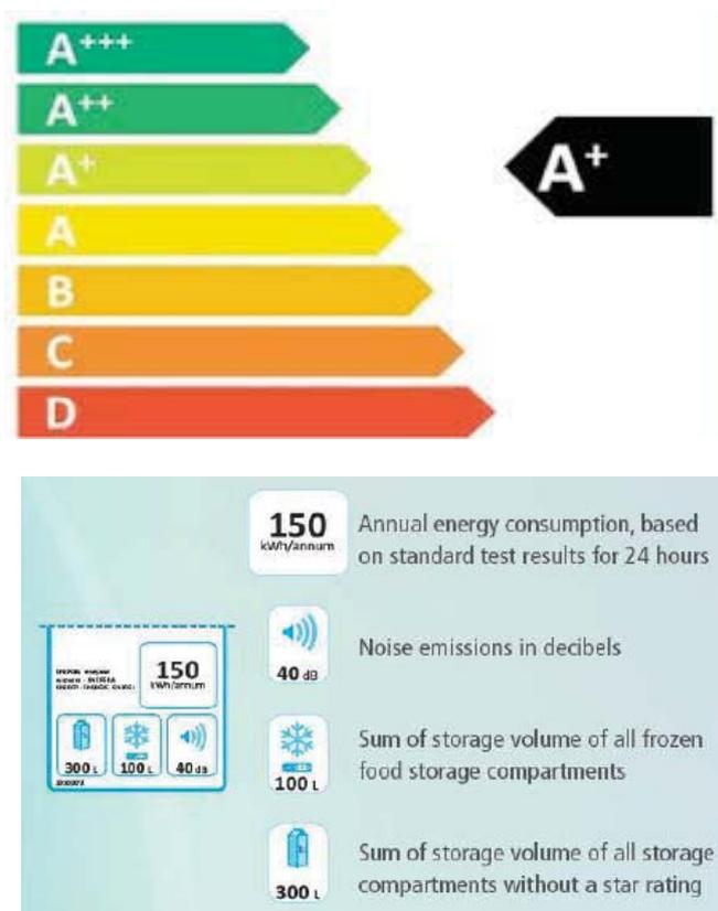
**Figure 9:** Draft for a new South African Energy Label (Example for Refrigerators)
